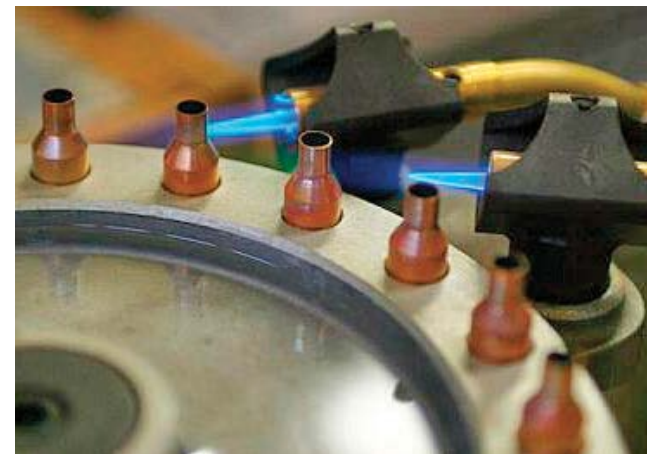
Jim DeKort home-built automated annealing machine
