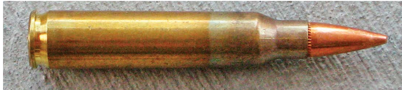
Discolouration on the neck and shoulder due to the annealing process
