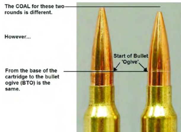
Two bullets with different ogive shapes, seated to the same CBTO, but having different COALs.
