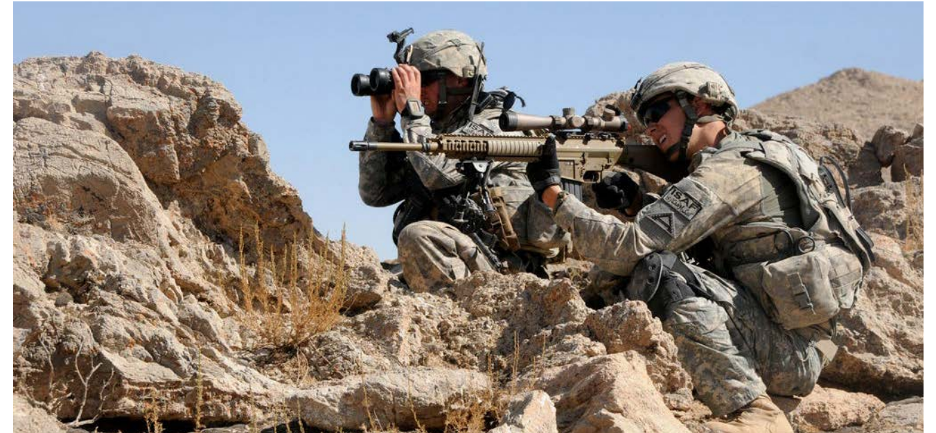
M110 semi-automatic sniper system. It shoots a 7.62x51mm round with an effective firing range of 866 yds.
