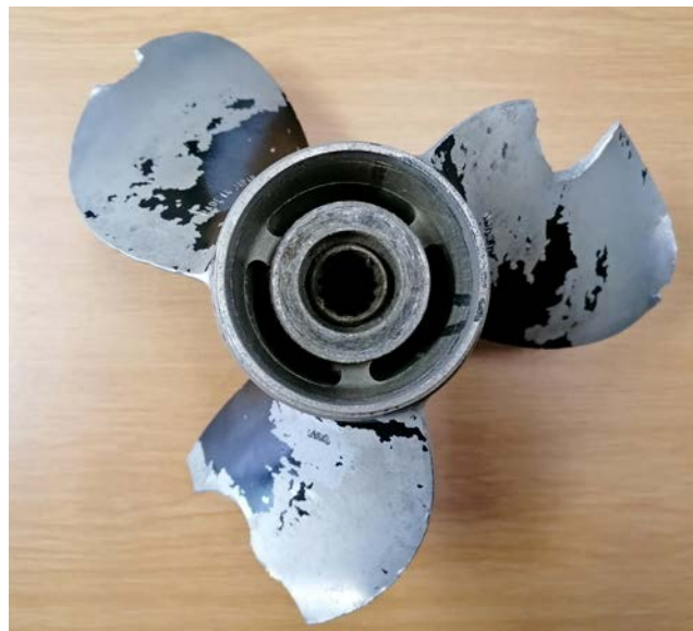
Damage done by the hippo to the boat's propeller.
